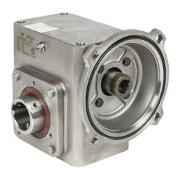
IronHorse heavy duty worm gearbox, 20:1 ratio, 56C-Face input, hollow, 1.4375in diameter output shaft, nominal 1.48hp at 1.0 SF, 907 lb-in mechanical output torque, 2-1/16in center distance, 304 stainless steel housing, top and bottom mount.
