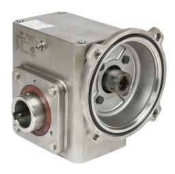
IronHorse heavy duty worm gearbox, 15:1 ratio, 56C-Face input, hollow, 1.4375in diameter output shaft, nominal 1.8hp at 1.0 SF, 850 lb-in mechanical output torque, 2-1/16in center distance, 304 stainless steel housing, top and bottom mount.
