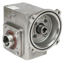
IronHorse heavy duty worm gearbox, 10:1 ratio, 56C-Face input, hollow, 1.4375in diameter output shaft, nominal 2.47hp at 1.0 SF, 799 lb-in mechanical output torque, 2-1/16in center distance, 304 stainless steel housing, top and bottom mount.
