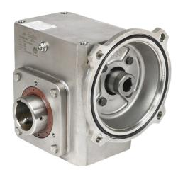
IronHorse heavy duty worm gearbox, 5:1 ratio, 56C-Face input, hollow, 1.4375in diameter output shaft, nominal 3.62hp at 1.0 SF, 640 lb-in mechanical output torque, 2-1/16in center distance, 304 stainless steel housing, top and bottom mount.
