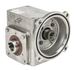
IronHorse heavy duty worm gearbox, 40:1 ratio, 56C-Face input, hollow, 1in diameter output shaft, nominal 0.57hp at 1.0 SF, 599 lb-in mechanical output torque, 1-3/4in center distance, 304 stainless steel housing, top and bottom mount.
