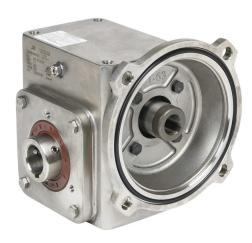
IronHorse heavy duty worm gearbox, 30:1 ratio, 56C-Face input, hollow, 1in diameter output shaft, nominal 0.65hp at 1.0 SF, 532 lb-in mechanical output torque, 1-3/4in center distance, 304 stainless steel housing, top and bottom mount.
