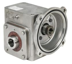
IronHorse heavy duty worm gearbox, 20:1 ratio, 56C-Face input, hollow, 1in diameter output shaft, nominal 0.85hp at 1.0 SF, 527 lb-in mechanical output torque, 1-3/4in center distance, 304 stainless steel housing, top and bottom mount.
