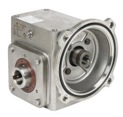
IronHorse heavy duty worm gearbox, 15:1 ratio, 56C-Face input, hollow, 1in diameter output shaft, nominal 1.09hp at 1.0 SF, 506 lb-in mechanical output torque, 1-3/4in center distance, 304 stainless steel housing, top and bottom mount.
