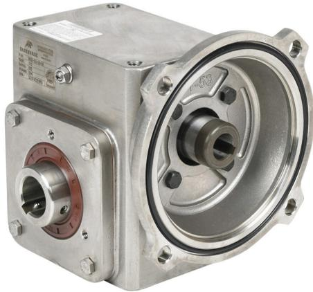
IronHorse heavy duty worm gearbox, 10:1 ratio, 56C-Face input, hollow, 1in diameter output shaft, nominal 1.52hp at 1.0 SF, 495 lb-in mechanical output torque, 1-3/4in center distance, 304 stainless steel housing, top and bottom mount.
