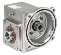
IronHorse heavy duty worm gearbox, 5:1 ratio, 56C-Face input, hollow, 1in diameter output shaft, nominal 2.36hp at 1.0 SF, 416 lb-in mechanical output torque, 1-3/4in center distance, 304 stainless steel housing, top and bottom mount.
