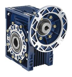
IronHorse medium-duty worm gearbox, 100:1 ratio, 56C-Face input, hollow, 1.25in diameter output shaft, nominal 0.75hp at 1.0 SF, 1593 lb-in mechanical output torque, 75mm center distance, cast aluminum housing, top and bottom mount.
