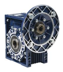
IronHorse medium-duty worm gearbox, 100:1 ratio, IEC 80B5 input, hollow, 28mm diameter output shaft, nominal 0.74hp at 1.0 SF, 1517 lb-in mechanical output torque, 75mm center distance, cast aluminum housing, top, bottom and back mount.
