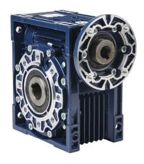
IronHorse medium-duty worm gearbox, 100:1 ratio, IEC 80B14 input, hollow, 28mm diameter output shaft, nominal 0.74hp at 1.0 SF, 1517 lb-in mechanical output torque, 75mm center distance, cast aluminum housing, top, bottom and back mount.
