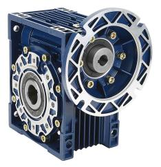
IronHorse medium-duty worm gearbox, 80:1 ratio, 56C-Face input, hollow, 1.25in diameter output shaft, nominal 0.75hp at 1.0 SF, 1672 lb-in mechanical output torque, 75mm center distance, cast aluminum housing, top and bottom mount.
