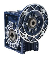
IronHorse medium-duty worm gearbox, 80:1 ratio, IEC 80B5 input, hollow, 28mm diameter output shaft, nominal 0.91hp at 1.0 SF, 1632 lb-in mechanical output torque, 75mm center distance, cast aluminum housing, top, bottom and back mount.
