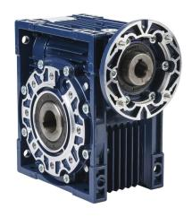
IronHorse medium-duty worm gearbox, 80:1 ratio, IEC 80B14 input, hollow, 28mm diameter output shaft, nominal 0.91hp at 1.0 SF, 1632 lb-in mechanical output torque, 75mm center distance, cast aluminum housing, top, bottom and back mount.
