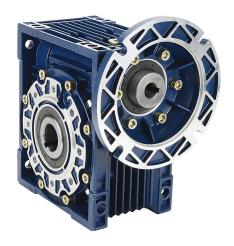
IronHorse medium-duty worm gearbox, 60:1 ratio, 56C-Face input, hollow, 1.25in diameter output shaft, nominal 1hp at 1.0 SF, 1770 lb-in mechanical output torque, 75mm center distance, cast aluminum housing, top and bottom mount.
