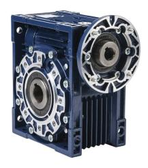
IronHorse medium-duty worm gearbox, 60:1 ratio, IEC 80B14 input, hollow, 28mm diameter output shaft, nominal 1.22hp at 1.0 SF, 1778 lb-in mechanical output torque, 75mm center distance, cast aluminum housing, top, bottom and back mount.
