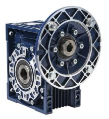
IronHorse medium-duty worm gearbox, 50:1 ratio, IEC 80B5 input, hollow, 28mm diameter output shaft, nominal 1.47hp at 1.0 SF, 1881 Ib-in mechanical output torque, 75mm center distance, cast aluminum housing, top, bottom and back mount.
