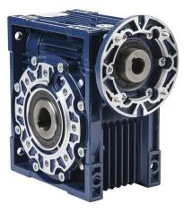
IronHorse medium-duty worm gearbox, 50:1 ratio, IEC 80B14 input, hollow, 28mm diameter output shaft, nominal 1.47hp at 1.0 SF, 1881 Ib-in mechanical output torque, 75mm center distance, cast aluminum housing, top, bottom and back mount.
