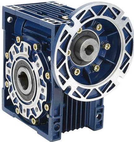
IronHorse medium-duty worm gearbox, 40:1 ratio, 56C-Face input, hollow, 1.25in diameter output shaft, nominal 1.5hp at 1.0 SF, 1947 lb-in mechanical output torque, 75mm center distance, cast aluminum housing, top and bottom mount.
