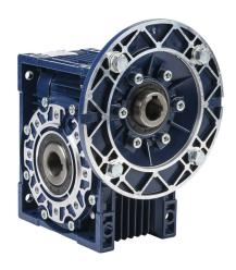
IronHorse medium-duty worm gearbox, 40:1 ratio, IEC 90B5 input, hollow, 28mm diameter output shaft, nominal 1.9hp at 1.0 SF, 2029 lb-in mechanical output torque, 75mm center distance, cast aluminum housing, top, bottom and back mount.
