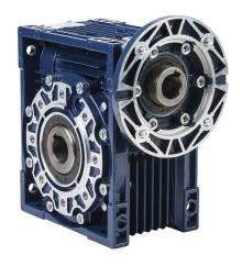
IronHorse medium-duty worm gearbox, 40:1 ratio, IEC 90B14 input, hollow, 28mm diameter output shaft, nominal 1.9hp at 1.0 SF, 2029 lb-in mechanical output torque, 75mm center distance, cast aluminum housing, top, bottom and back mount.
