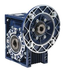
IronHorse medium-duty worm gearbox, 40:1 ratio, IEC 80B5 input, hollow, 28mm diameter output shaft, nominal 1.9hp at 1.0 SF, 2029 lb-in mechanical output torque, 75mm center distance, cast aluminum housing, top, bottom and back mount.
