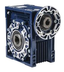
IronHorse medium-duty worm gearbox, 40:1 ratio, IEC 80B14 input, hollow, 28mm diameter output shaft, nominal 1.9hp at 1.0 SF, 2029 lb-in mechanical output torque, 75mm center distance, cast aluminum housing, top, bottom and back mount.
