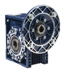
IronHorse medium-duty worm gearbox, 30:1 ratio, IEC 90B5 input, hollow, 28mm diameter output shaft, nominal 2.41hp at 1.0 SF, 2028 lb-in mechanical output torque, 75mm center distance, cast aluminum housing, top, bottom and back mount.
