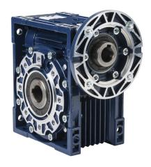
IronHorse medium-duty worm gearbox, 30:1 ratio, IEC 90B14 input, hollow, 28mm diameter output shaft, nominal 2.41hp at 1.0 SF, 2028 lb-in mechanical output torque, 75mm center distance, cast aluminum housing, top, bottom and back mount.
