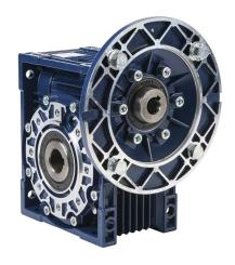
IronHorse medium-duty worm gearbox, 30:1 ratio, IEC 80B5 input, hollow, 28mm diameter output shaft, nominal 2.41hp at 1.0 SF, 2028 lb-in mechanical output torque, 75mm center distance, cast aluminum housing, top, bottom and back mount.
