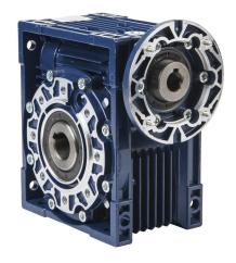
IronHorse medium-duty worm gearbox, 30:1 ratio, IEC 80B14 input, hollow, 28mm diameter output shaft, nominal 2.41hp at 1.0 SF, 2028 lb-in mechanical output torque, 75mm center distance, cast aluminum housing, top, bottom and back mount.
