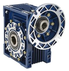
IronHorse medium-duty worm gearbox, 20:1 ratio, 145TC-Face input, hollow, 1.25in diameter output shaft, nominal 3hp at 1.0 SF, 1849 lb-in mechanical output torque, 75mm center distance, cast aluminum housing, top and bottom mount.
