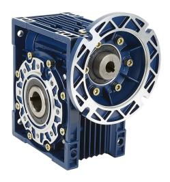
IronHorse medium-duty worm gearbox, 20:1 ratio, 56C-Face input, hollow, 1.25in diameter output shaft, nominal 3hp at 1.0 SF, 1849 lb-in mechanical output torque, 75mm center distance, cast aluminum housing, top and bottom mount.
