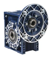
IronHorse medium-duty worm gearbox, 20:1 ratio, IEC 90B5 input, hollow, 28mm diameter output shaft, nominal 3.24hp at 1.0 SF, 1953 lb-in mechanical output torque, 75mm center distance, cast aluminum housing, top, bottom and back mount.
