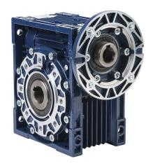
IronHorse medium-duty worm gearbox, 20:1 ratio, IEC 90B14 input, hollow, 28mm diameter output shaft, nominal 3.24hp at 1.0 SF, 1953 lb-in mechanical output torque, 75mm center distance, cast aluminum housing, top, bottom and back mount.
