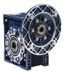
IronHorse medium-duty worm gearbox, 20:1 ratio, IEC 80B5 input, hollow, 28mm diameter output shaft, nominal 3.24hp at 1.0 SF, 1953 Ib-in mechanical output torque, 75mm center distance, cast aluminum housing, top, bottom and back mount.
