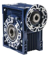
IronHorse medium-duty worm gearbox, 20:1 ratio, IEC 80B14 input, hollow, 28mm diameter output shaft, nominal 3.24hp at 1.0 SF, 1953 Ib-in mechanical output torque, 75mm center distance, cast aluminum housing, top, bottom and back mount.
