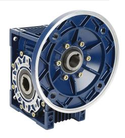
IronHorse medium-duty worm gearbox, 10:1 ratio, 182/4TC-Face input, hollow, 1.25in diameter output shaft, nominal 5hp at 1.0 SF, 1717 lb-in mechanical output torque, 75mm center distance, cast aluminum housing, top and bottom mount.
