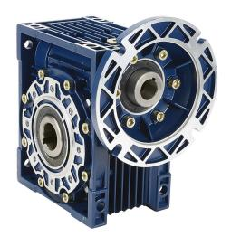
IronHorse medium-duty worm gearbox, 10:1 ratio, 145TC-Face input, hollow, 1.25in diameter output shaft, nominal 5hp at 1.0 SF, 1717 lb-in mechanical output torque, 75mm center distance, cast aluminum housing, top and bottom mount.
