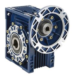
IronHorse medium-duty worm gearbox, 10:1 ratio, 56C-Face input, hollow, 1.25in diameter output shaft, nominal 5hp at 1.0 SF, 1717 lb-in mechanical output torque, 75mm center distance, cast aluminum housing, top and bottom mount.
