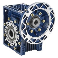
IronHorse medium-duty worm gearbox, 100:1 ratio, 56C-Face input, hollow, 1.125in diameter output shaft, nominal 0.5hp at 1.0 SF, 1035 lb-in mechanical output torque, 63mm center distance, cast aluminum housing, top and bottom mount.
