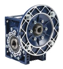
IronHorse medium-duty worm gearbox, 100:1 ratio, IEC 80B5 input, hollow, 25mm diameter output shaft, nominal 0.51hp at 1.0 SF, 992 lb-in mechanical output torque, 63mm center distance, cast aluminum housing, top, bottom and back mount.
