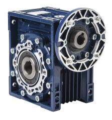
IronHorse medium-duty worm gearbox, 100:1 ratio, IEC 80B14 input, hollow, 25mm diameter output shaft, nominal 0.51hp at 1.0 SF, 992 lb-in mechanical output torque, 63mm center distance, cast aluminum housing, top, bottom and back mount.
