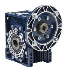
IronHorse medium-duty worm gearbox, 100:1 ratio, IEC 71B5 input, hollow, 25mm diameter output shaft, nominal 0.51hp at 1.0 SF, 992 lb-in mechanical output torque, 63mm center distance, cast aluminum housing, top, bottom and back mount.
