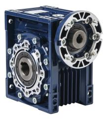
IronHorse medium-duty worm gearbox, 100:1 ratio, IEC 71B14 input, hollow, 25mm diameter output shaft, nominal 0.51hp at 1.0 SF, 992 lb-in mechanical output torque, 63mm center distance, cast aluminum housing, top, bottom and back mount.
