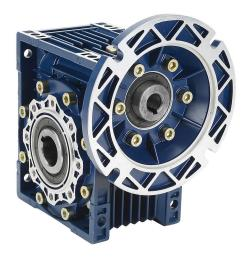
IronHorse medium-duty worm gearbox, 80:1 ratio, 56C-Face input, hollow, 1.125in diameter output shaft, nominal 0.5hp at 1.0 SF, 1071 lb-in mechanical output torque, 63mm center distance, cast aluminum housing, top and bottom mount.
