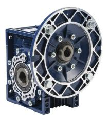
IronHorse medium-duty worm gearbox, 80:1 ratio, IEC 80B5 input, hollow, 25mm diameter output shaft, nominal 0.6hp at 1.0 SF, 1027 Ib-in mechanical output torque, 63mm center distance, cast aluminum housing, top, bottom and back mount.
