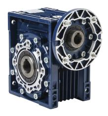
IronHorse medium-duty worm gearbox, 80:1 ratio, IEC 80B14 input, hollow, 25mm diameter output shaft, nominal 0.6hp at 1.0 SF, 1027 lb-in mechanical output torque, 63mm center distance, cast aluminum housing, top, bottom and back mount.
