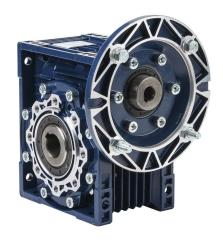
IronHorse medium-duty worm gearbox, 80:1 ratio, IEC 71B5 input, hollow, 25mm diameter output shaft, nominal 0.6hp at 1.0 SF, 1027 lb-in mechanical output torque, 63mm center distance, cast aluminum housing, top, bottom and back mount.
