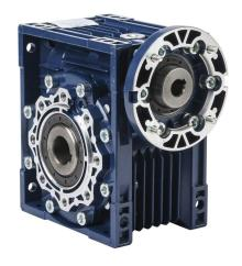
IronHorse medium-duty worm gearbox, 80:1 ratio, IEC 71B14 input, hollow, 25mm diameter output shaft, nominal 0.6hp at 1.0 SF, 1027 lb-in mechanical output torque, 63mm center distance, cast aluminum housing, top, bottom and back mount.
