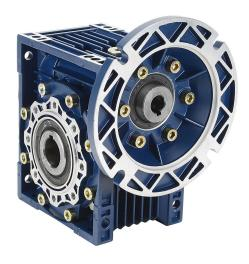
IronHorse medium-duty worm gearbox, 60:1 ratio, 56C-Face input, hollow, 1.125in diameter output shaft, nominal 0.75hp at 1.0 SF, 1141 lb-in mechanical output torque, 63mm center distance, cast aluminum housing, top and bottom mount.
