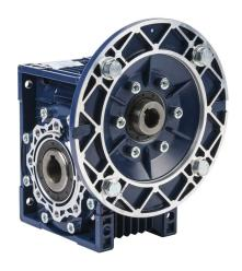
IronHorse medium-duty worm gearbox, 60:1 ratio, IEC 80B5 input, hollow, 25mm diameter output shaft, nominal 0.82hp at 1.0 SF, 1135 lb-in mechanical output torque, 63mm center distance, cast aluminum housing, top, bottom and back mount.
